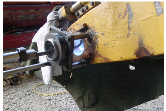
Orbital Welding Of A 100mm Ø Bore On a Digger Bucket
