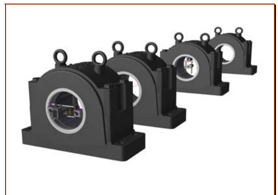
Laser Bore Alignment
